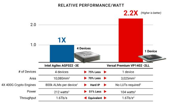
Intel Agilex I series device with 200G half-duplex crypto was not available in the tools
