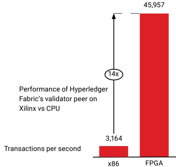
The Varium C1100 card is based on Xilinx UltraScale+. Estimated results are based on Intel Xeon Silver 4114 vs Xilinx UltraScale+ transactions / sec.
