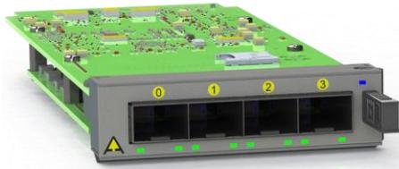
Fig. 8: Aperi FPGA-based Micro Server Hardware
